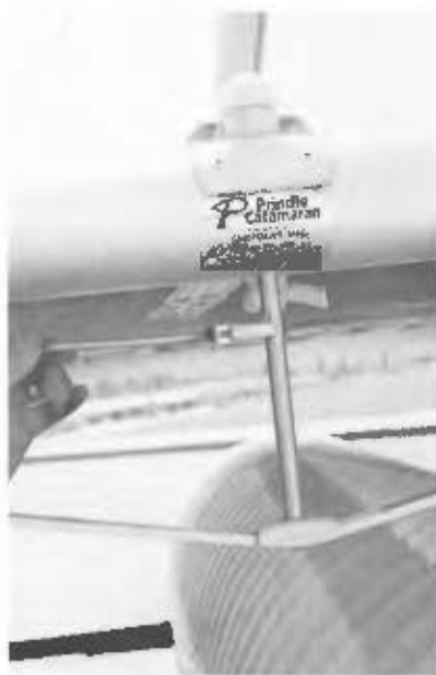
Loosen screw at bottom of striker rod.
