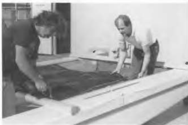
Slide the rear piece and zip the two pieces together.
