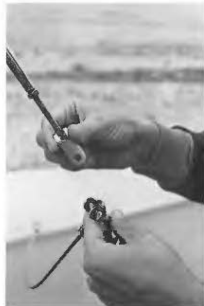
Raise the mast to your shoulder and walk forward with it while extending arms over your head until the mast is held by the side shrouds.
