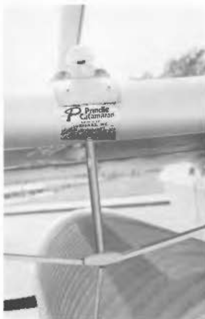
Loosen screw at bottom of striker rod.
