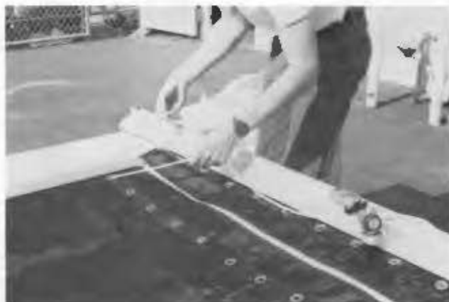
Slide the sides down each side of the trampoline track. Two people are needed here.
