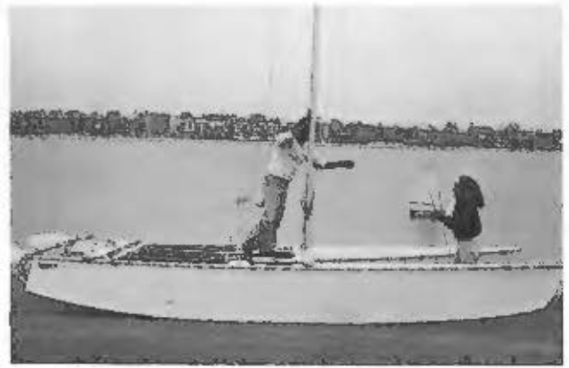
Raise the mast to your shoulder and walk forward with it while extending arms over your head until the mast is held by the side shrouds.
