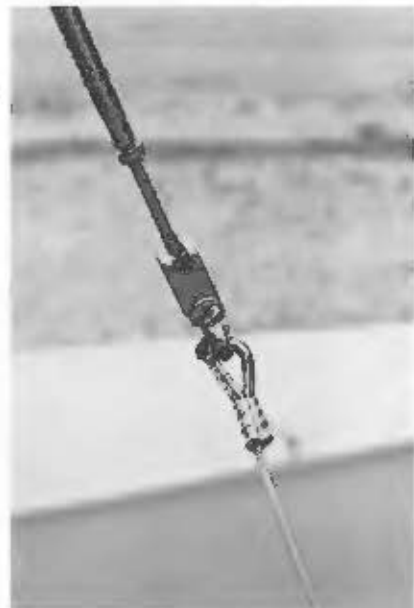
Attach the forestay to the 1/4" shackle holding the bow bridle wires together. After the initial rigging,
