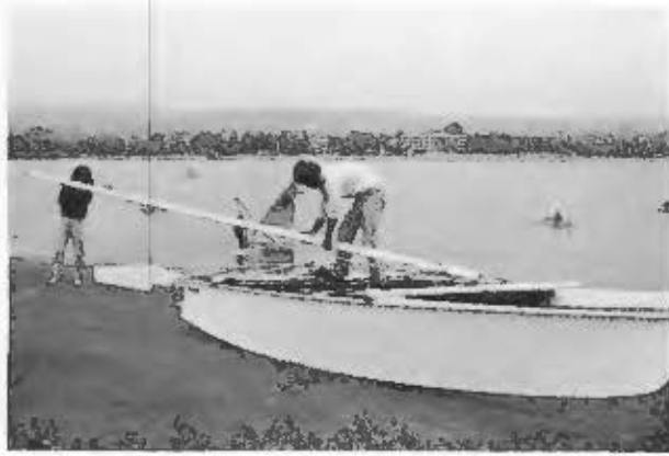
Stand on trampoline with one foot on rear cross-bar to steady yourself.
